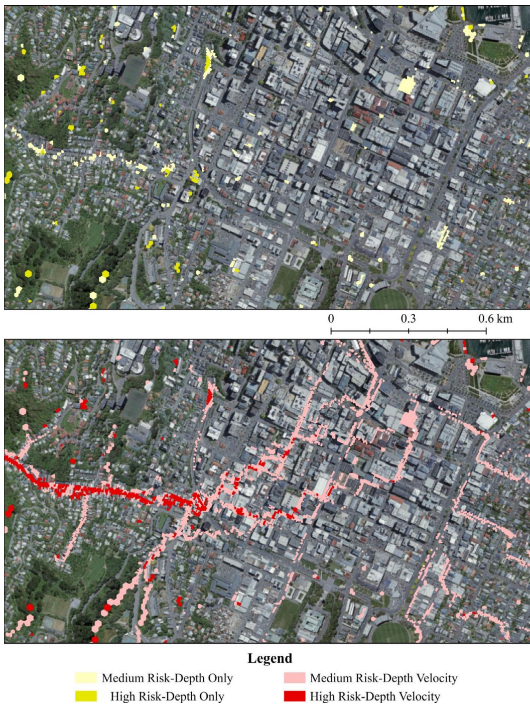
FIGURE 7 | Pedestrian high and medium depth-only and depth-velocity risk maps at rainfall peak time (16h).
